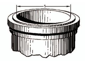
The end gaps expand depending on the liner bore and for each 0.03 mm (0.001 inch) increase in the cylinder liner bore size, the clearance between the ends of the piston ring increases by 0.08 mm (0.003 inch).
