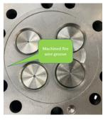
Cylinder Head Modifications: IPD cautions the use of our raised edge liner in conjunction with modified cylinder heads. One of the more common modifications shops are doing to the cylinder head is cutting a receiving groove in the surface of the head for a secondary fire wire. There are no consistent specs for the diameter or depth of the grooves the machine shops are making into the head, so it's unknown if these modifications will conflict with the raised edges of our liners.
