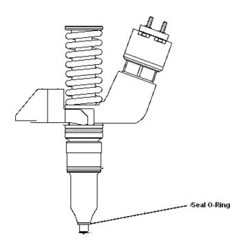
The function of the seal O-ring at the tip of these injectors is to seal long enough during the break in period for a "carbon dam" to be established. Once the "carbon dam" is in place the seal O-ring has serviced its purpose and due to the harsh conditions associated to this area of the engine the O-ring will deteriorate. This is a normal occurrence and does not affect the engine's performance or cause the injector to fail.
