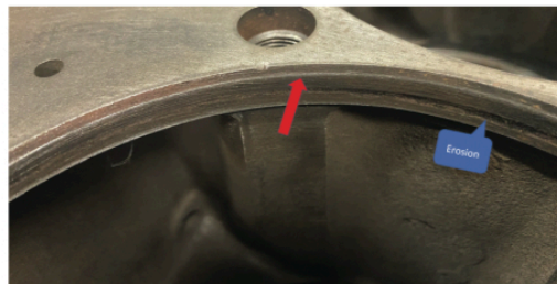
Examples of wear found around the circumference in the upper receiver bores of a high mileage ISX block.
