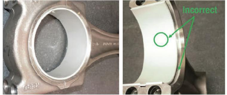
**Bearing Installed Incorrectly – the oil port is blocked and the bearing is not evenly centered in the rod.**
