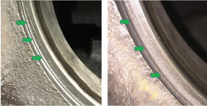
If the counter bore height, or if depth variance is greater than is 0.025mm (0.001") and/or the surface of the counter bore ledge is beyond the reusability guidelines, the block will need to be machined for a repair shim.
