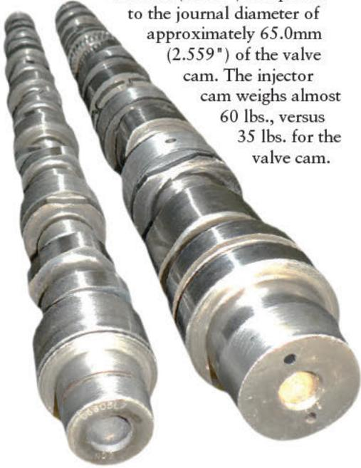
While it may be common practice to drive the camshaft bushing in for other engines, Cummins installation instructions indicate that the cam bushings (injector and valve) are to be pressed in (not driven). Several cylinder head rebuilders have reported that they are convinced that due to the size and amount of retention (crush) holding the injector cam bushings in place, they cannot be driven in without distorting or damaging the bushing, resulting in bushing failures.
