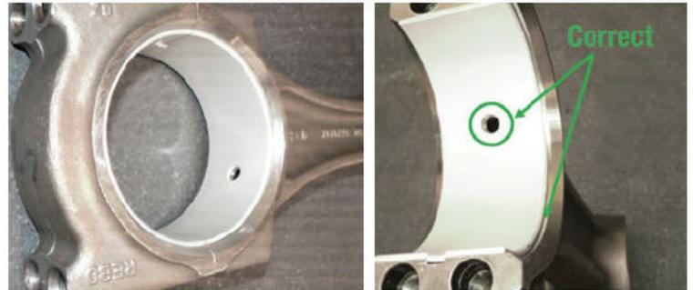
**Bearing Installed Correctly – the oil port is open and the bearing is evenly centered in the rod.**
