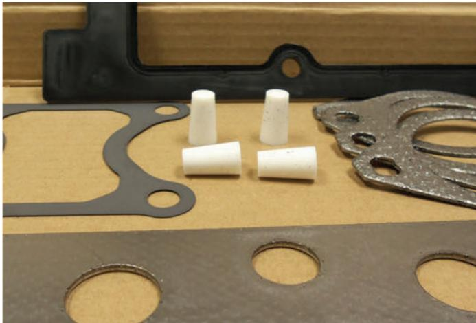
Over the years, Cummins has had various service campaigns and literature stressing the importance of using these plugs during repairs on ISX engines. Sadly, these plugs are often overlooked.
