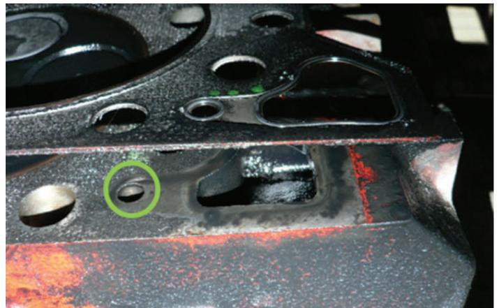
Of course, there are far more ports and openings to consider on an engine than just where these plugs are used. In fact, there are additional plugs used for the front and sides of the cylinder block. The OE service manuals have more detailed instructions for keeping debris out, and for cleaning and protecting engine components.
