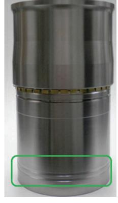
and two grooves (bands) on the APR liner that are visible on the outside bottom of each liner that identifies them as being one of the bronze shim designs. Those grooves (shown above) do not identify the diameter of the liner, so, the cylinder block and liner must be measured to assure they are a correct fit.
