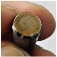
surfaces between the valve and seat (insert). The valve of the right is more prone to be held slightly open and not allowed to seal properly. Either condition can cause a valve to overheat. Over time, most valves will develop the dimple in the center of the tip from normal wear. Comparing wear patterns between components is a good process to follow.
