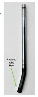
valve can also allow hot combustion gasses to coke(burn) the oil film in the guide. The coking of oil means that is has become glass like and no longer aids in the transfer of heat and becomes an insulator. As the carbon build-up produced is very abrasive, coupled with its inability to transfer heat, the components wear quickly. Carbon and excessive wear are
