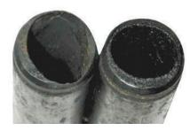
very visible in photo of two valve guides shown here. The next question is if the guide is the cause or the result.
