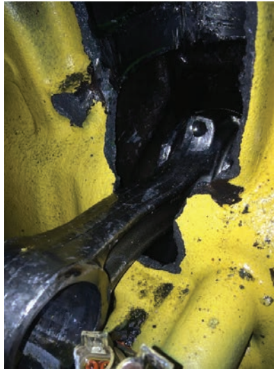
Connecting rod through the side of the block, metal debris, damaged piston coolers, and RTV sealant blocking oil stream.
