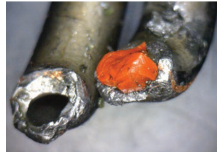
Connecting rod through the side of the block, metal debris, damaged piston coolers, and RTV sealant blocking oil stream.
