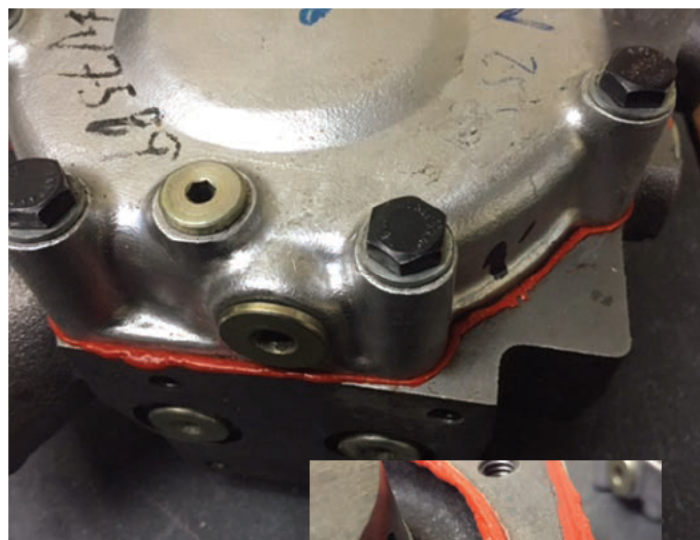
Self-applied sealant goes inside crankcase.
