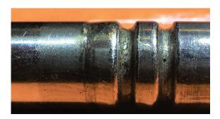
The keeper grooves in this photo are rounded over, and there is significant damage on the stem from the valve locks. This would not be a candidate for reuse.
