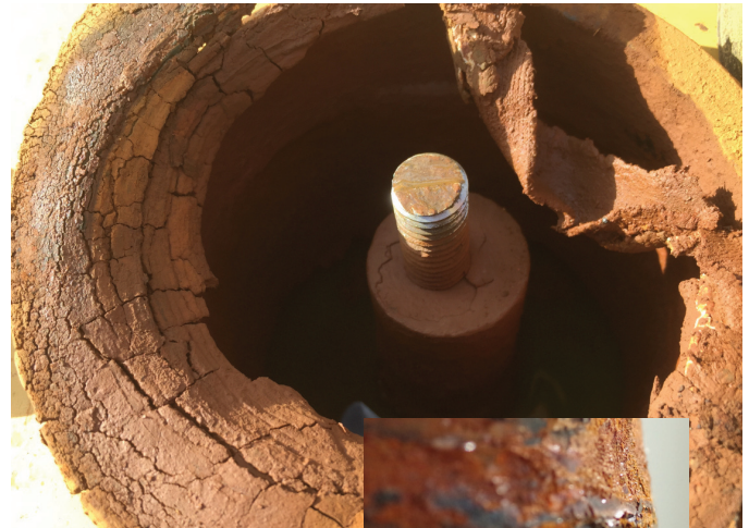
Scale is a barrier that blocks heat transfer. 1/16" of scale build up reduces heat transfer by approximately 40%.
