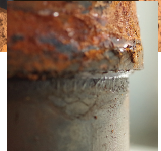
Cylinder liner pitting (cavitation) is a chemical and physical occurrence that results in pitting of the outside of cylinder liners. In extreme instances, these pits will travel through the liner and into the combustion cylinder.
