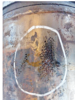
Cylinder liner pitting (cavitation) is a chemical and physical occurrence that results in pitting of the outside of cylinder liners. In extreme instances, these pits will travel through the liner and into the combustion cylinder.
