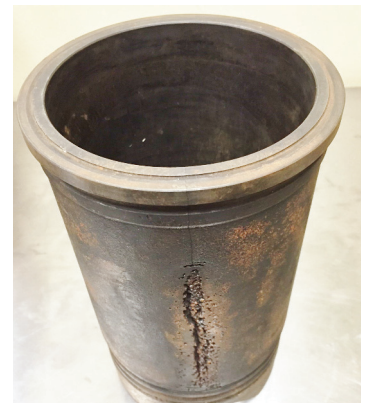
Cylinder liner pitting (cavitation) is a chemical and physical occurrence that results in pitting of the outside of cylinder liners. In extreme instances, these pits will travel through the liner and into the combustion cylinder.
