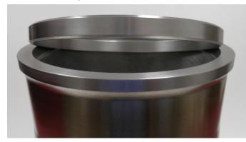
While in the engine, these liners can be identified by the two bands machined around the bottom of the liner. Mixing an APR liner with non-APR liners within an engine is not recommended.
