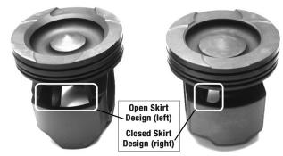
One piece pistons must be used with drilled connecting rods and rod bearings. Failure to align the deep valve pocket and the piston skirt cooling notch correctly will result in extensive engine damage. Refer to the latest OE service bulletin or contact IPD for further information.
