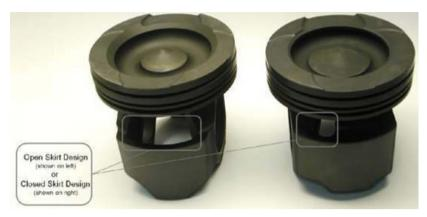
o Care must be taken when replacing less than full septis tofn s within an engine since the actual piston design may have updateidn wanit hengine kit previously installed. Examples:
