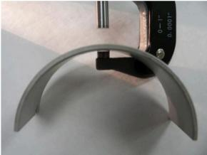
Micrometers with pointed or blade anvils and dial calipers should not be used as they can give false readings and damage the bearing surface. Obviously using an accurate, recently calibrated micrometer is a must for reliable measurement.
