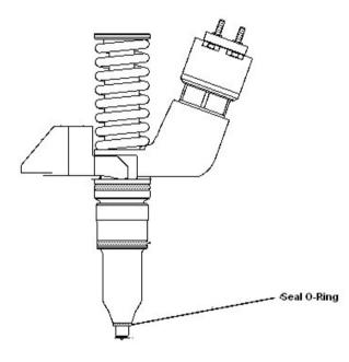
The function of the seal O-ring at the tip of these injectors is to seal long enough during
