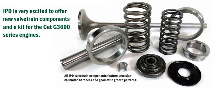
**FEATURES:** IPD offers a wide range of quality, precision-engineered engine repair parts. The G3600 features a shot-peened exhaust valve to ensure superior strength. Both intake and exhaust valves have induction-hardened tips. The exhaust valve seat (face) features a cobalt-chromium alloy hardface for ultimate high temperature wear resistance.
