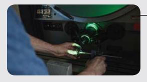
Shown here is our in-house tangential piston ring tension tester.
