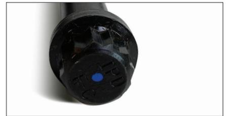
Each cryo-treated head bolt has a blue dot on its head so that you know it's been cryo- treated.
