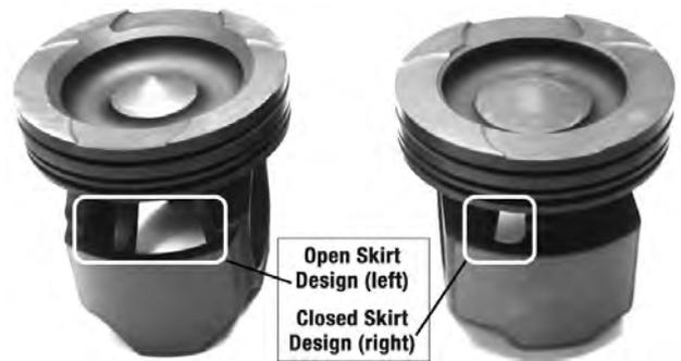
One piece pistons must be used with drilled connecting rods and rod bearings. Failure to align the deep valve pocket and the piston skirt cooling notch correctly will result in extensive engine damage. Refer to the latest OE service bulletin or contact IPD for further information.
