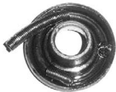
Photo at left shows excessive spring wear resulting in breakage of spring and bearing after only 40,000 miles into second service life of part.
